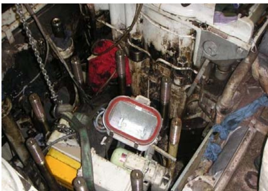
The crane mechanism lying on top of the engine.
