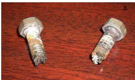
Photo 3. Two of the failed bolts. The other two had similarly failed.
