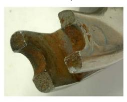
Fracture surfaces on port shackle. Note the corrosion especially in the bore of the holes for the pin.
