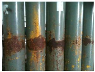
The remaining air bottles, showing the corrosion in the area where the retaining strap had been fitted.
