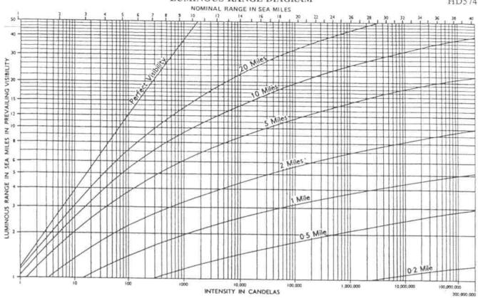
Luminous Range Diagram.—This diagram enables the mariner to determine the approximate range at which a light may be sighted, at night, in the meteorological visibility prevailing at the time of observation.
